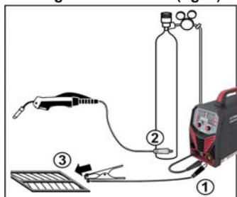
Welding with flux-cored wire (Figure 2)
