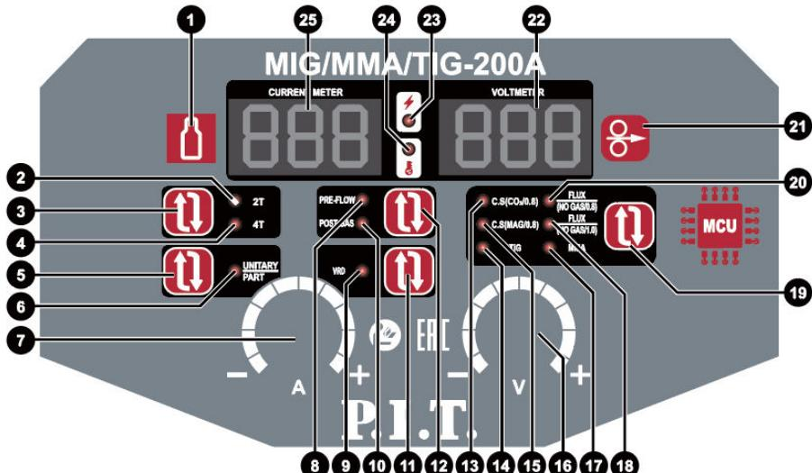
1. Gas check function: check whether the gas is connected to the machine and whether there is gas out of the welding torch
