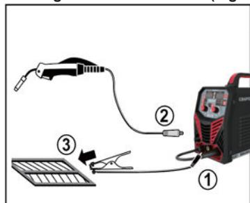
Welding with an electrode (Figure 3)
