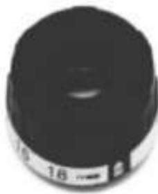
When screwing of screws in different materials, you can adjust the rotational moment. The regulator ring has a scale from 0 to 18 plus drilling mode. To set the desired figure, combine the digit on the regulator ring with the arrow on the case top.
